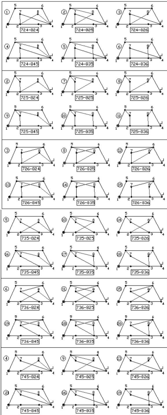
Figure 5. Enumeration results for independent link connection
