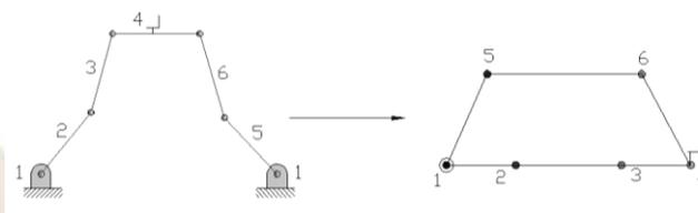
Figure 1. Linkage diagram of a planar parallel robot and its corresponding Graphical representation
