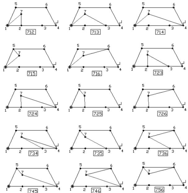
Figure 3. Fifteen arrangements for 1<sup>st</sup> step in independent link connection
