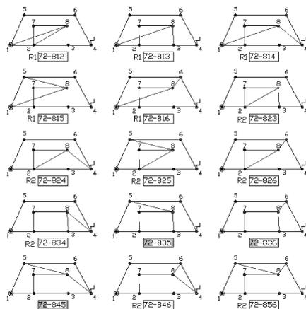
Figure 11. Fifteen available structures for arrangement "72" of dependent link
