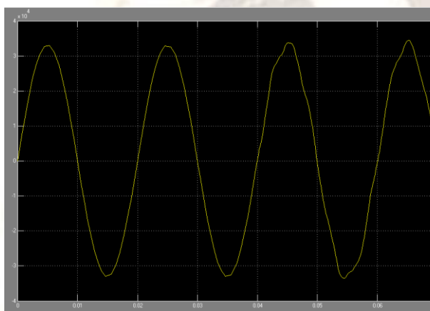
Fig.19.Oscillatory voltage appearing at MX1 transformer terminal. Switching time(0.04).
