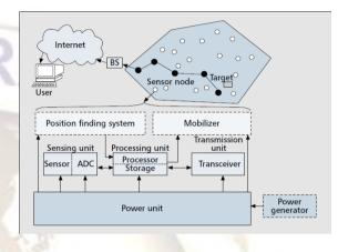
Figure 1. The components of a sensor node
