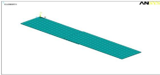
Fig 2 Meshed geometry of single spot welded specimen
