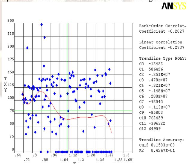
Fig.6 scattered plot of shear stress Vs thickness distribution of spot welded specimen.
