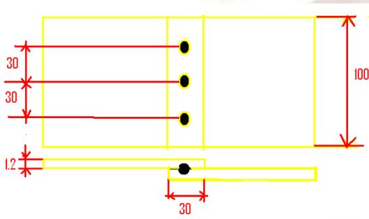
Fig.3.Dimensions of tensile-shear test specimen with three spot (not to scale, dimensions in mm).
