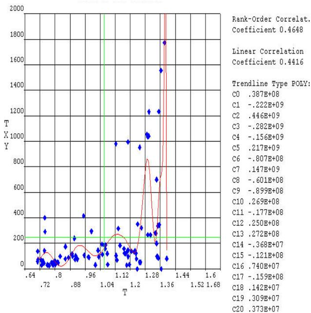
Fig.7 scattered plot of shear stress Vs thickness distribution of three spot welded specimen.
