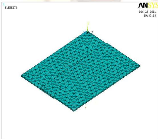
Fig.4 Meshed geometry of three spot welded specimen
