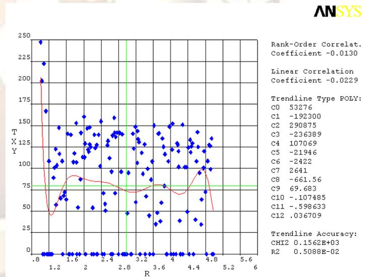
Fig.9 scattered plot of shear stress Vs radius for single spot welded specimen
