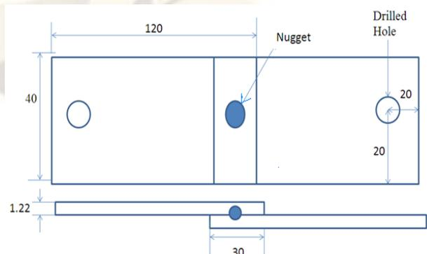
Fig.1. Dimensions of single spot lap shear tensile-shear test specimens (not to scale, dimensions in mm).
