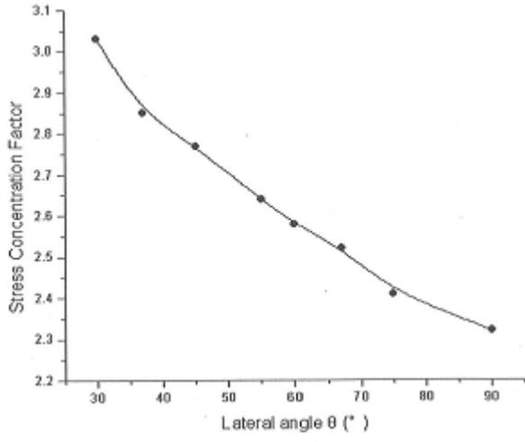
Fig. 6 Influence of lateral angle  $\theta$  on SCF (on acute side of cylinder)
