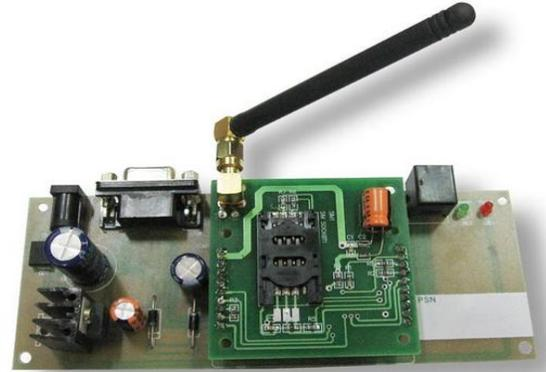
Figure.5. GSM modem
