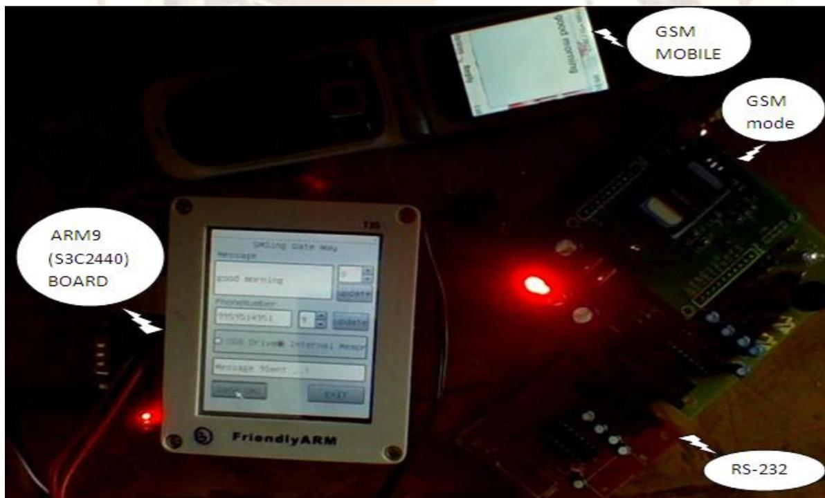
Figure. 5 Sending data from ARM9 board to mobile
