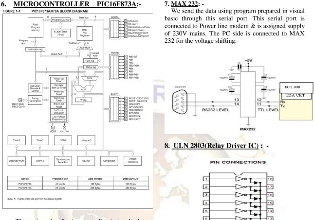
The main role of microcontroller is to check received information with the prepared program available inside the microcontroller; depending upon which several relays (i.e. devices) are operated.
