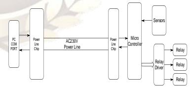
**3.1 <u>Functional Description</u>:-** In this Project the data is being transferred over AC line from PC communication port, which is encoded and decoded by PLC chips. The received information signal is then send to the microcontroller and according to the
