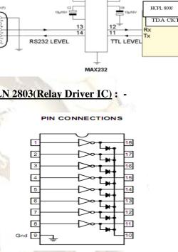
The eight NPN Darlington connected transistors in this family of arrays are ideally suited for interfacing between low logic level digital circuitry (such as TTL, CMOS or PMOS/NMOS) and the higher current/voltage requirements of lamps, relays, printer hammers or other similar loads for a broad range of computer, industrial, and consumer applications. All devices feature open-collector outputs and freewheeling clamp diodes for transient suppression.
