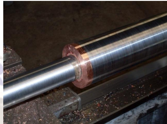
Figure 1.4 A typical squirrel cage rotor for submersible motor being machined (Courtesy VIRA PUMPS)
