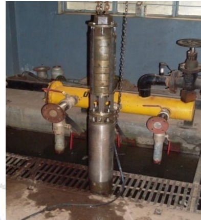
Figure 1.9 5 HP Motor coupled with 8 stage Radial type Submersible pump (Courtesy: VIRA PUMPS)
