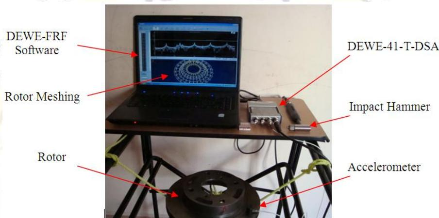
Figure 2. Experimental Modal Analysis set-up
