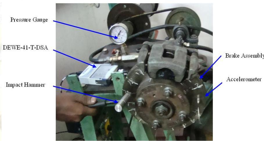
Figure 4. Experimental modal analysis of disc brake assembly.
